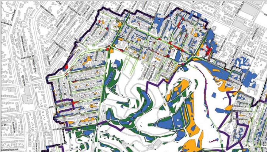
Figure showing SUSTAIN output of "GIS Features" that identify possible locations for potential "BMP Feature" within a portion of the Nine Mile Run Sewershed
